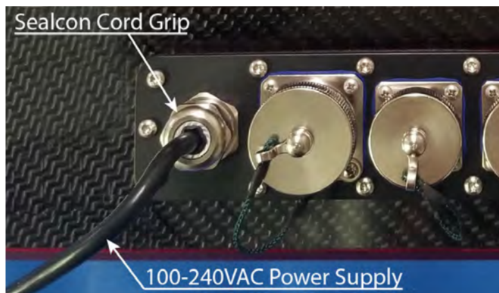
Figure 31 — Power Supply connected through Sealcon Cord Grip
