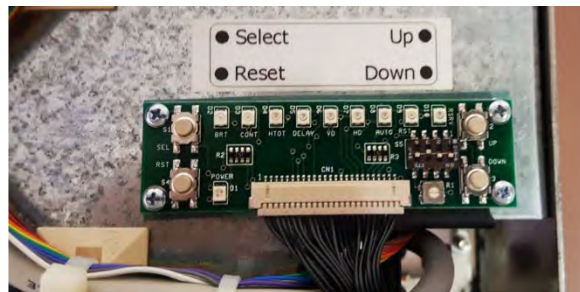
Figure 4 – External OSD Controller
